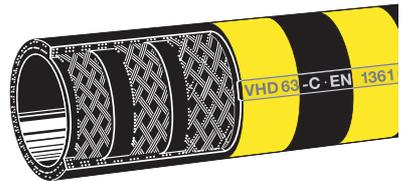
Special type "VHD" with three textile braids and thicker wall for lower bending radii and good suction rates. Burst pressure > 100 bar/1500 psi.
