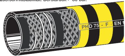
Special type "PHD" with non metallic semihard polyamide helix and thick wall for enhanced lateral stability. Burst pressure > 80 bar/1200 psi.
