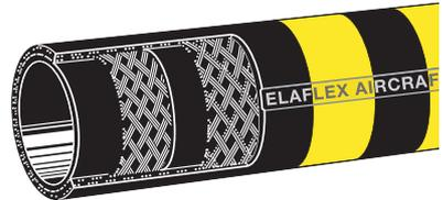
**"Yellow Band"** aircraft refuelling hoses, suitable for all aviation gasolines and jet fuels (JET A 1), deicing fluids and motor oils. Temperature range -30° up to +70° Celsius. Electrical resistance between 10<sup>3</sup> and 10<sup>6</sup> Ohm.
